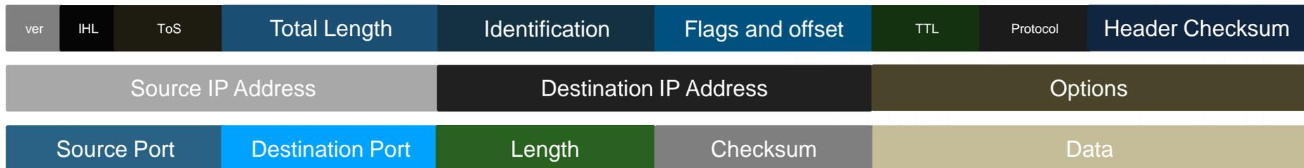
\*IPv4 Packet (IPv6 header is bigger)
